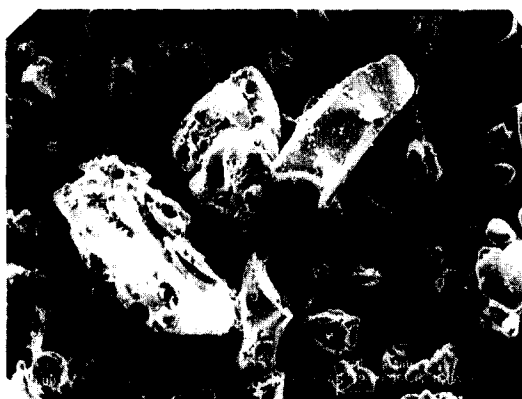
Fig. 3. SEM photomicrograph of pure GL.
